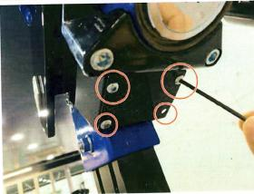
Place **Bottom Plate** beneath and line up all holes.
