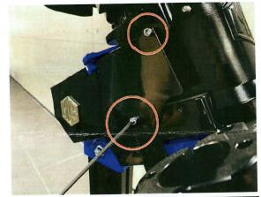
Tuck the wire harness and clutch cable, brake line under the **Neck Cover Side Plate.**
