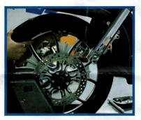
Begin by installing your wheel bearing removal tool in a way that it will only capture the ABS sensor spacer and not the whole bearing itself. With the tool installed on the wheel follow the instructions to remove the bearing.
