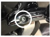
2. Remove four inner fairing bolts using a T25 Torx driver. Two inner fairing bolts are located below each glove box, adjacent to each wind deflector. Store these screws in a safe place for installation later.
