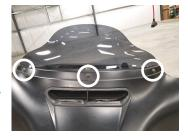
2. Remove four inner fairing bolts using a T27 Torx screw driver. The four inner fairing bolts are located adjacent to each turn indicator mounting bracket and below/adjacent to each speaker. Store these screws in a safe place for re-installation later.
