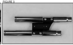
Remove the muffler assemblies and heat shields from their protective packaging. Place each heat shield on a nonabrasive surface such as a towel, blanket or carpet.
