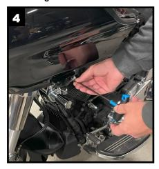
Remove both left and right lower T-25 torx bolts from the bottom of each fairing chin spoiler. Shown in Figure 5.
