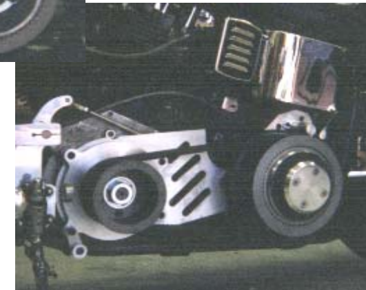
KIT IS SHOWN WITH OPTIONAL SLOTTED GREAT PLATE, ALTERNATOR COVER WITH TIMING MARKS, 3" BELT DRIVE WITH PRO-CLUTCH AND BILLET REAR PULLEY COVER.
